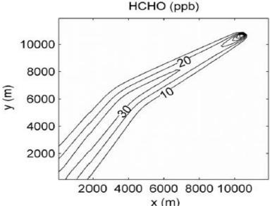
Concentration isopleths of ozone (upper figure) and formaldehyde (lower figure) generated by a large olefin flare after 3 hours (9 am – 12 pm, LST) of constant flare emissions, as simulated by Olaguer (2012) at **200 m** resolution.
