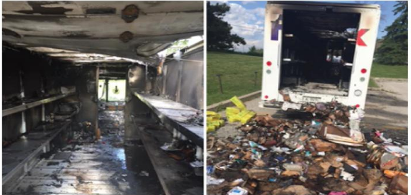
The damage resulting from a lithium-ion battery fire in a FedEx truck is shown in these photos taken June 2, 2016. Left: The fire damage to the FedEx truck and its contents. Right: The contents of the truck were removed by firefighters following the fire. Photos courtesy of FedEx.
